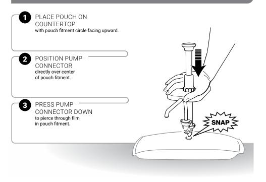
Pump is fully engaged when top surface of pouch fitment touches pump connector rim.
