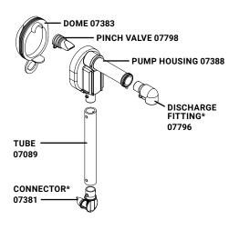
1 INSERT PINCH VALVE into pump housing.
