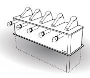
Drop-in units can be used either on a countertop surface or can be dropped into an opening in a countertop.
