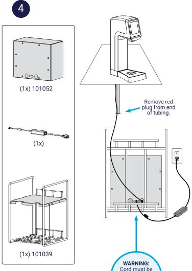
plugged into the unit first, before plugging into an outlet.
