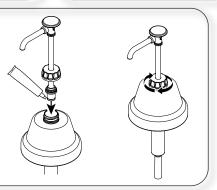
8 Insert pump into product container. Prime pump by continuously pressing on the pump until any air bubbles are eliminated and only product is dispensed.
