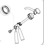
Install stop collar onto side of head assembly piston. Add optional gaging collar(s) to reduce portion size.
