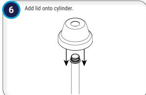
Install head assembly in cylinder. Apply small amount of food equipment lubricant inside top of cylinder and outside of seal. Slide locking collar down onto cylinder threading. Tighten firmly.
