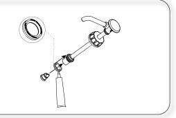
Install stop collar onto side of head assembly. Optional: Add gaging collars to reduce portion size.
