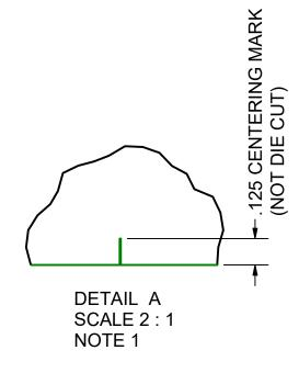
NOTE 1: THE PROTECTIVE BACKING MUST HAVE A VERTICAL SLIT IN LOCATION SHOWN. THE VISIBLE FACE MUST HAVE A CENTERING MARK FOR ALIGNMENT PURPOSES IN LOCATION SHOWN.
