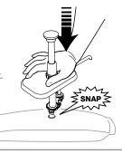
Pump is fully engaged when top surface of pouch fitment touches pump connector rim.
