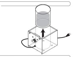
**PULL REMOVABLE BOTTOM** out from slot at base of shroud.
