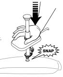
Pump is fully engaged when top surface of pouch fitment touches pump connector rim.
