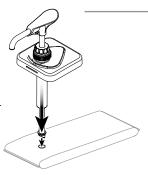
Pump connector is fully engaged when top surface of pouch fitment touches pump connector rim.
